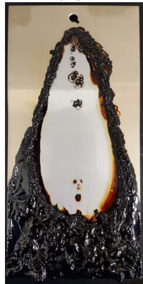
Closed Coke Pattern Failed at 230°C
