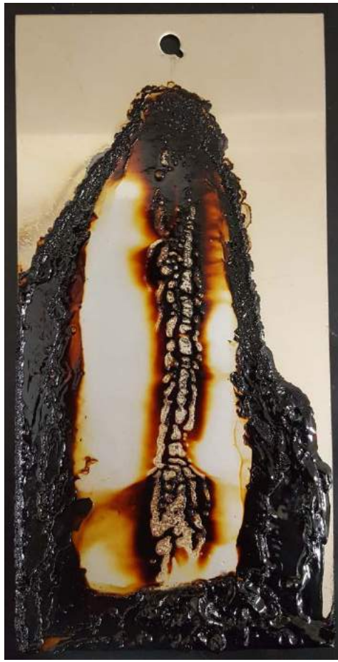
Closed Coke Pattern 90% Group III 10% AN-19
