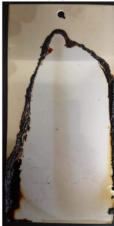
Open Coke Pattern Passed at 220°C
