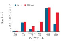
SpectraSyn Elite 300 provides good shear stability.
