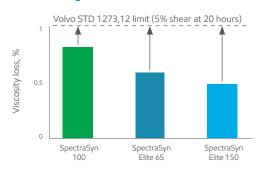
The shear stability benefits of SpectraSyn Elite mPAOs can translate into finished formulations.
