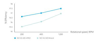
SpectraSyn Elite 150 can provide enhanced energy efficiency in formulated oils compared to mineral oils.
