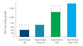
SpectraSyn Elite mPAOs provide the ability to blend to a wide viscosity range.
