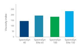
SpectraSyn Elite mPAOs demonstrate improved viscosity index.
