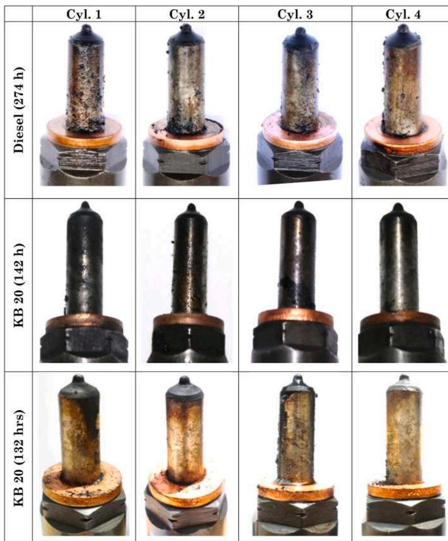
Fig. 6. Carbon deposits on the injectors of KB20 and diesel-fuelled engines.
