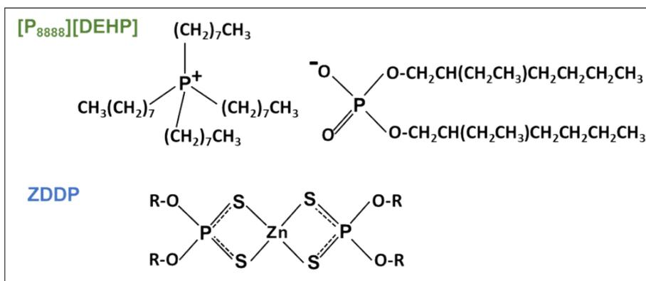
Figure 1. Chemical structures of  $[P_{8888}][DEHP]$  and ZDDP. R represents an alkyl group and typically range from C4-C12
