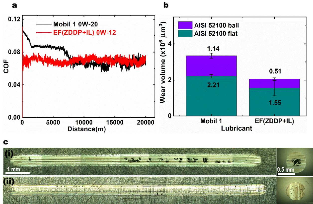
**Figure 6.** Friction traces (a) and wear volumes (b) of self-mate AISI 52100 contacts lubricated with EF(ZDDP+IL) and Mobil 1 0W-20 oils at 100 °C for 20 km. (c) Wear scars morphology of the AISI 52100 steel ball and flat lubricated with (i) Mobil 1 0W-20 and (ii) EF(ZDDP+IL), at 100 °C.
