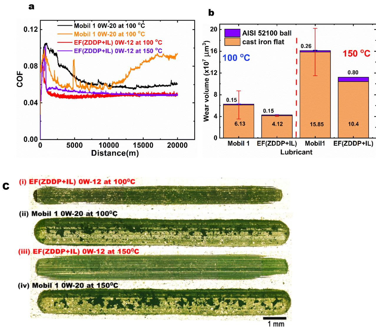
Figure 3. Friction traces (a) and wear volumes of the cast iron flats (b) lubricated by Mobil 1 0W-20 and EF (ZDDP+IL) at 100 and 150 °C. (c) Wear scar morphology of the cast iron flat lubricated by (i) EF(ZDDP+IL), (ii) Mobil 1 0W-20 at 100 °C, (iii) EF(ZDDP+IL) at 150 °C, and (iv) Mobil 1 0W-20 at 150 °C.
