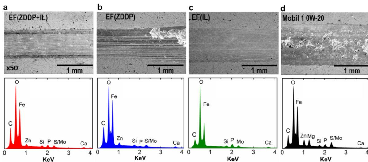
**Figure 4.** Wear scar SEM images and EDS spectra of the cast iron flats lubricated by (a) EF(ZDDP+IL), (b) EF(ZDDP), (c) EF(IL), and (d) Mobil 1 0W-20.
