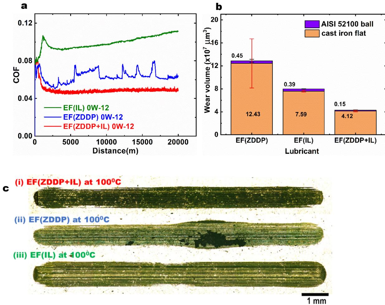
**Figure 2.** Friction traces (a) and wear volumes of the cast iron flats (b) lubricated by EF(ZDDP), EF(IL), and EF(ZDDP+IL) at 100 °C. (c) Wear scar morphology of the cast iron flat lubricated by (i) EF(ZDDP+IL), (ii) EF(ZDDP), and (iii) EF(IL) at 100 °C.
