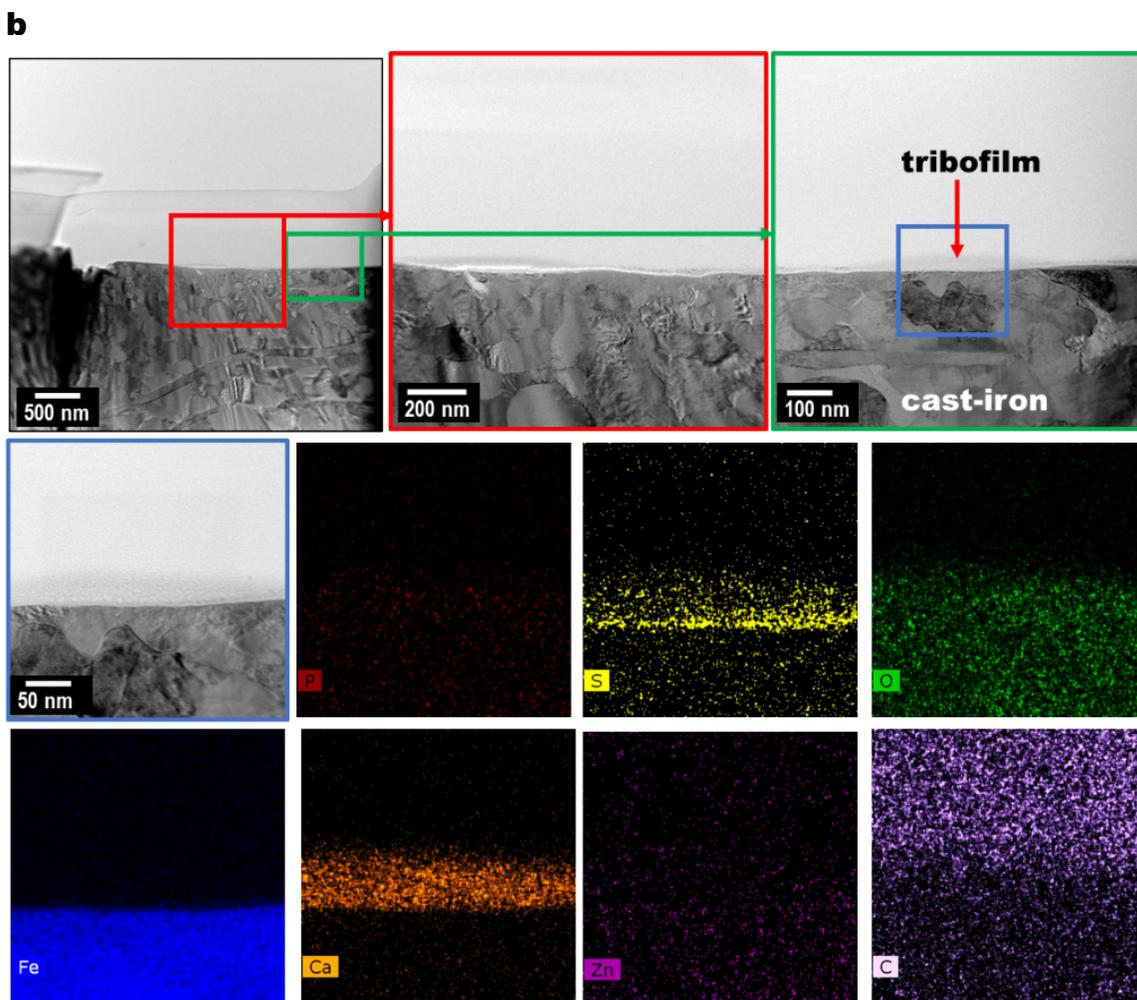
**Figure 5.** Cross-sectional STEM images and EDS elemental maps of the tribofilms on the cast iron flats lubricated by (a) EF(ZDDP+IL) and (b) Mobil 1 0W-20 at 100 °C for 20 km.
