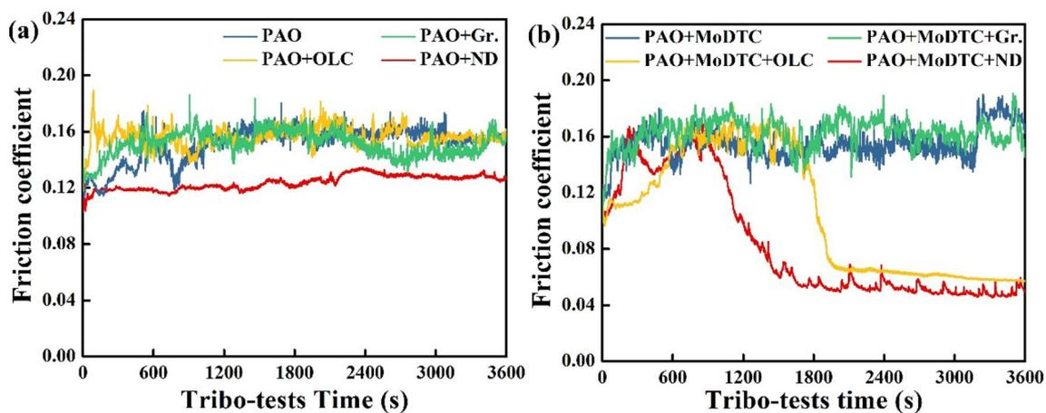
**Fig. 6** Effects of nano-carbon materials on friction coefficient of self-mated AISI52100 steels lubricated under PAO oil **a** without and **b** with Mo-DTC additive
