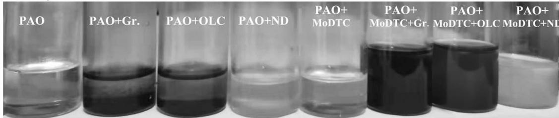
**Fig. 5** Results of settlement observations showing the dispersion of PAO oil with suspended nano-carbon and MoDTC additives
