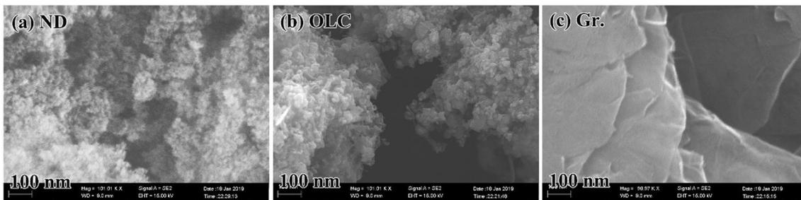
Fig. 3 SEM images showing the morphologies of a ND, b OLC and c graphene additives
