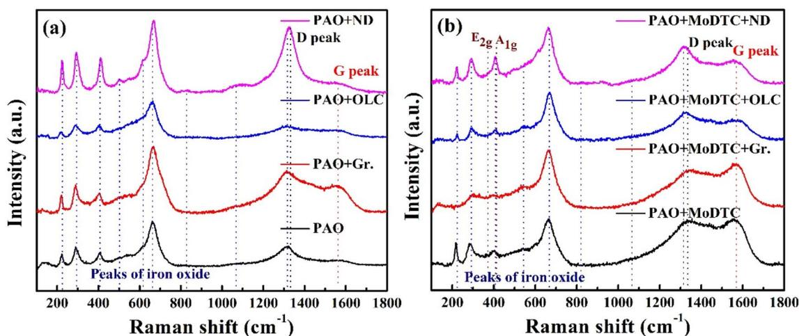
Fig. 11 Raman spectra of worn surfaces of the disc lubricated under PAO oil with a individual nano-carbon and b both MoDTC and nano-carbon additives
