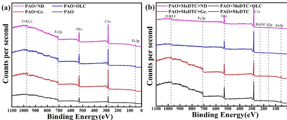
**Fig. 13** XPS analysis of the worn surfaces of the disc lubricated under PAO oil with **a** individual nano-carbon and **b** both MoDTC and nano-carbon additives
