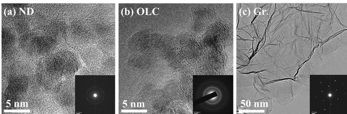
Fig. 4 HR-TEM images and SAED patterns of a ND, b OLC and c graphene additives
