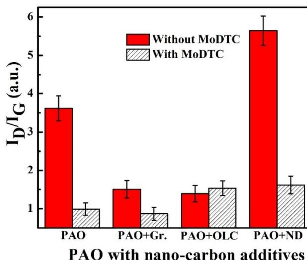
Fig. 12 The ratios of D peak intensity to G peak intensity ( $I_D/I_G$ ) of Raman spectra for the disc lubricated under PAO oil with MoDTC and nano-carbon additives
