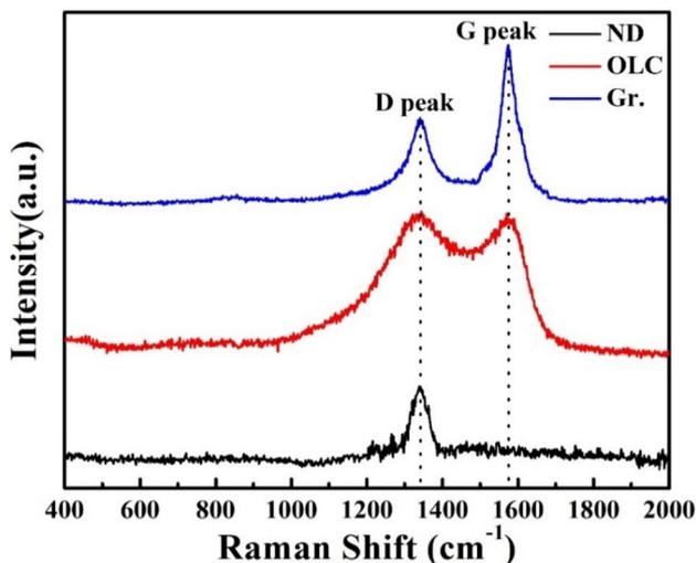
Fig. 2 Raman spectra of ND, OLC and graphene additives
