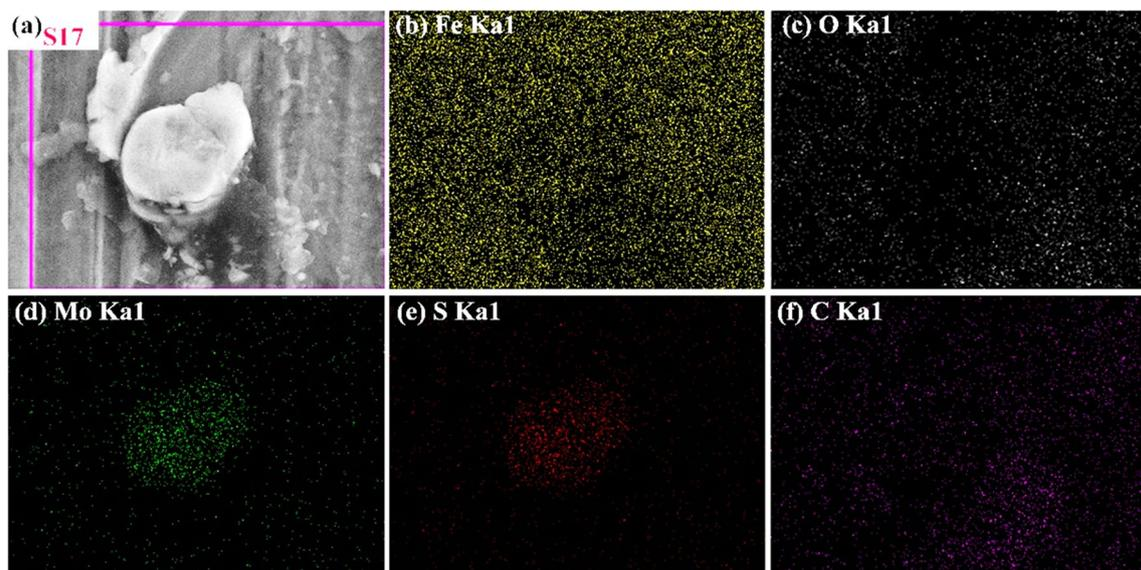
**Fig. 10** EDS surface spectrum showing the distribution of elements on worn surface of the disc lubricated under PAO oil with MoDTC and ND additives: **a** SEM image showing the spectrum area via pink rectangle and **b–f** the distribution maps of Fe, O, Mo, S and C
