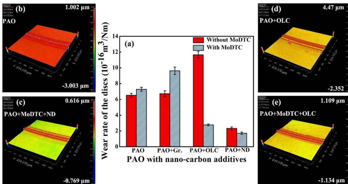
**Fig. 7** Anti-wear performances of PAO oil with nano-carbon and MoDTC additives shown via **a** wear rates and **b–e** worn surface 3D morphologies of AISI52100 discs
