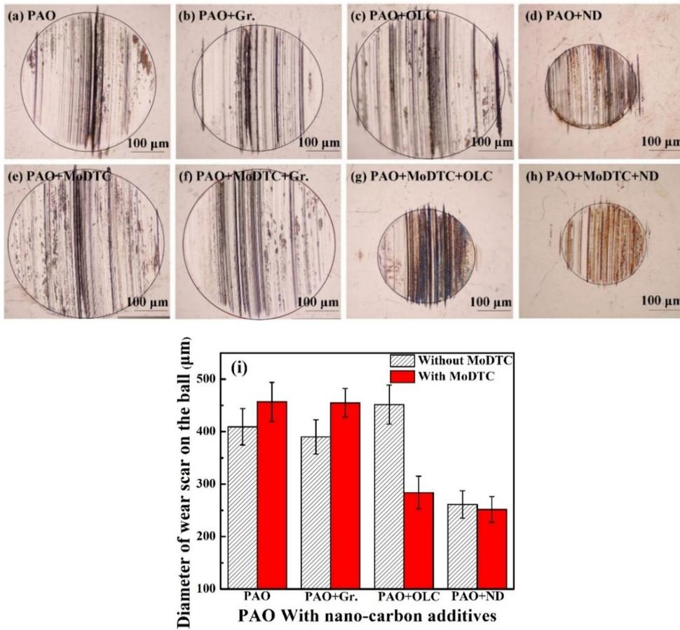
**Fig. 8** Wear behaviors of the AISI52100 steel lubricated under PAO oil with nano-carbon and MoDTC additives shown via **a–h** surface morphology and **i** diameter of wear scar
