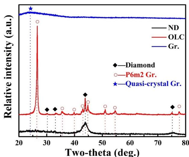
Fig. 1 XRD patterns of ND, OLC and graphene additives
