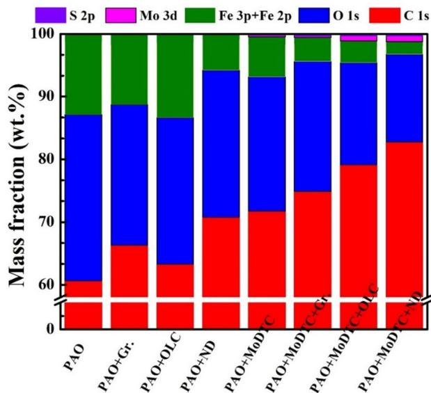
**Fig. 14** Chemical elemental composition of worn surface on the discs lubricated under PAO oil with MoDTC and ND additives
