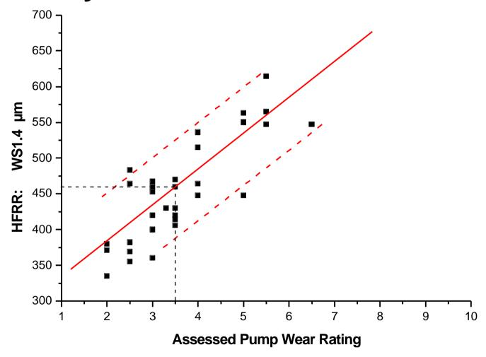
→ Linear regression: Pump wear 3.5 ==> WS1.4 = 454 µm
