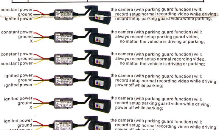
never power on; X means no connection or connect to ground
