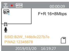
2. Enter the smartphone WLAN(Wi-Fi) settings menu, select the B2W dash camera SSID: B2W\_xxxxxx and enter the password 12345678 to continue.
