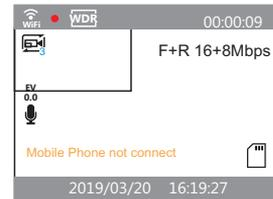
6. Long press the Down button to disable Wi-Fi function on camera. The Wi-Fi icon will be locked, and camera will be back to standard video recording mode automatically.
