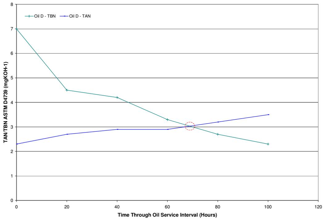
Figure 3 Fresh Oil TBN vs Maximum Oil Drain Capability
