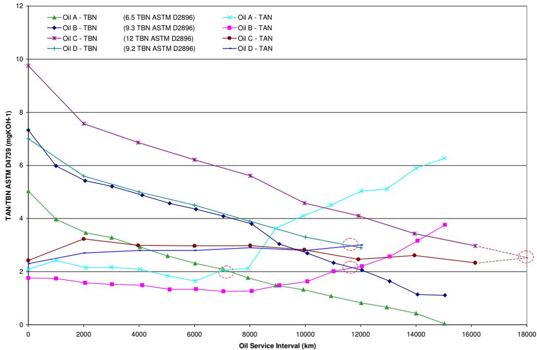
Figure 2 TAN/TBN vs Test Time (Dynamometer)
