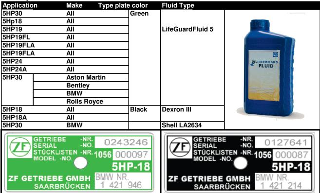
Type plate examples see above for correct transmission - type plate color - fluid type
