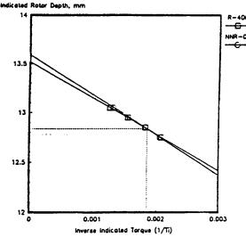
FIG. 4 Reciprocal Torque Intercept Method for Setting Appropriate Rotor Position
