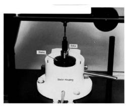
FIG. 2 Rotor, Stator, and Stator Housing
