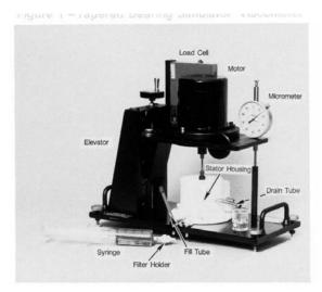
FIG. 1 Tapered Bearing Simulator-Viscometer
