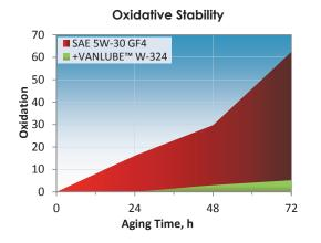
**HTCBT\*** Corrosion TEST \*165°C, 0-72h; 750 ppm W ASTM D7214 FTIR Oxidation
