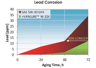
HTCBT\* Corrosion TEST \*165°C, 0-72h; 750 ppm W ICP Analysis
