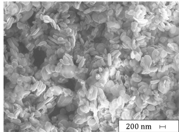
**Fig. 4.** SEM image of the nano hBN particles.
