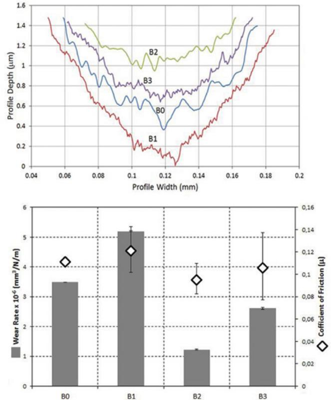
**Fig. 7.** Wear profiles, the specific wear rates and the coefficient of friction of samples. (Figure available in color online.)
