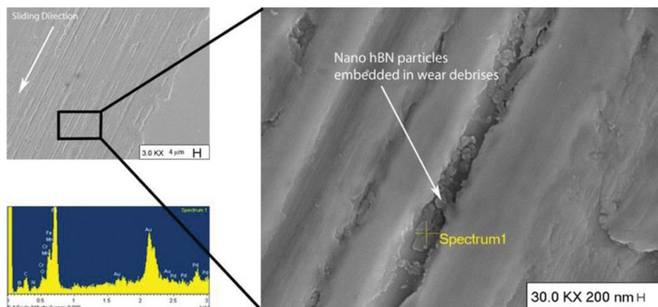
**Fig. 6.** The wear track, the wear debris and the chemical analysis of the wear debris for sample B2. (Figure available in color online.)
