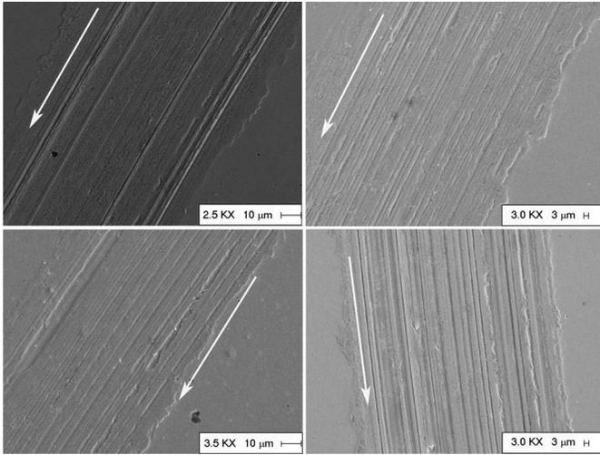
**Fig. 8.** SEM images of worn surfaces of discs using different lubricants: (a) B0, (b) B1, (c) B2 and (d) B3.
