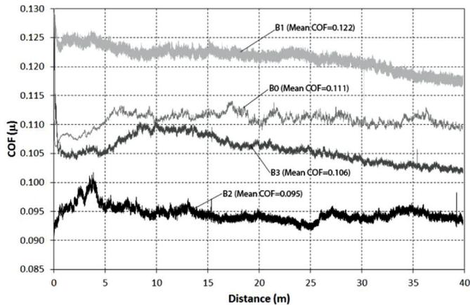
**Fig. 5.** Coefficients of friction as functions of the sliding distance (2.5 cm/s sliding speed).
