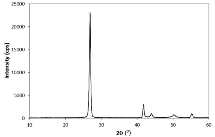
**Fig. 3.** XRD pattern of the nano hBN powder.
