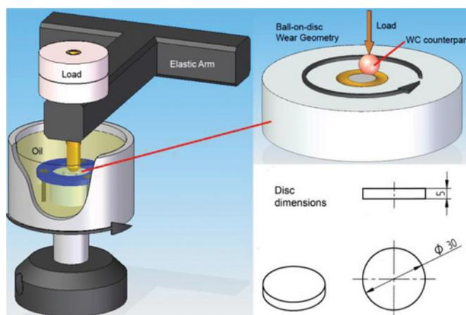
**Fig. 1.** A schematic wear test device, the wear geometry and the disc dimensions. (Figure available in color online.)
